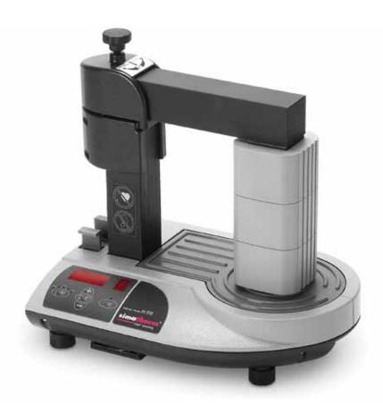
The medium-sized simatherm induction heater for roller bearings and other circular metal workpieces up to 400 mm bore diameter and a cross section of 145 x 205 mm. With the integrated time and temperature controls, roller bearings can be heated to the prescribed 110°C while other circular metal workpieces can be heated to 400°C.
