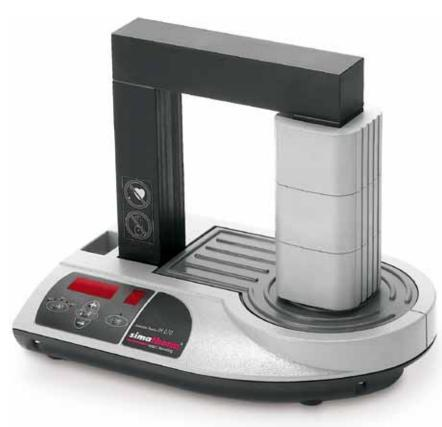
The medium-sized simatherm induction heater for roller bearings and other circular metal workpieces up to 400 mm bore diameter and a cross section of 145 x 205 mm. With the integrated time and temperature controls, roller bearings can be heated to the prescribed 110°C while other circular metal workpieces can be heated to 400°C.
